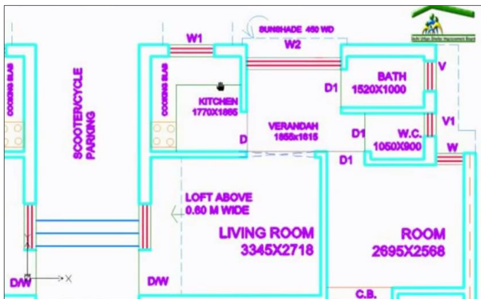
ONE COMPLETE UNIT OF EWS HOUSING (Source: http://delhishelterboard.in/main/?page_id=3644 )
